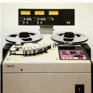
APR-5003 The APR-5003 IEC center track time code version is specially targeted to meet the requirements of broadcasters and post production houses. Featuring the ability to generate, record and reproduce a time code track in the "guard band" found on NAB standard 2-track recordings, the APR-5003 is ideal for lock up to VTR's or other ATR's. The AutoLocator readouts on this machine show time code in hours, minutes, seconds and frames. AutoLocate routines can be performed accurately to time code addresses. Microprocessor intelligence ensures the coincidence of code to recorded/reproduced audio, and serial control capability makes the APR-5003 ideal for integration into video editing systems.
