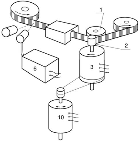
*Fig. 6: Weber and Augustin: Synchronisation between film and magnetic tape by means of "sprockets" printed on the back of the tape<sup>31</sup>*
