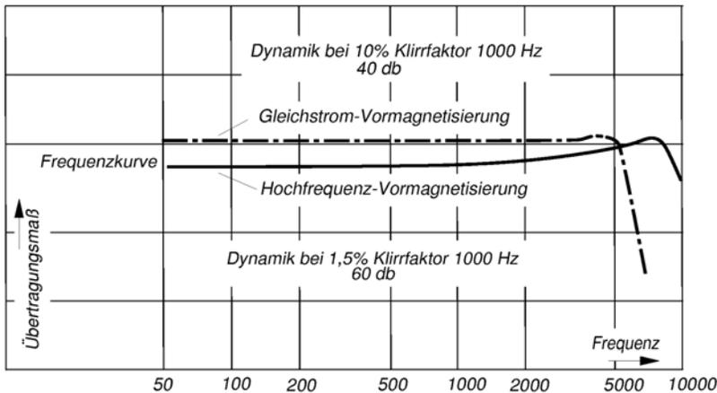
Fig. 3: Frequency response and dynamic with DC bias ("Gleichstrom-Vormagnetisierung") und AC bias ("Hochfrequenz-Vormagnetisierung"), showing also a significant reduction of distortions from 10 % to 1.5 %<sup>18</sup>
