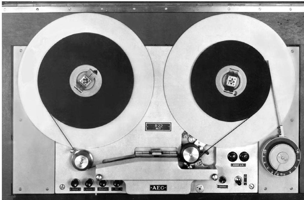
Fig. 5: Magnetic tape recorder "Magnetophon R 22" of about 1939, customer built by AEG for RRG (German Radio). Tape speed 77 cm/s (approx. 30 ips), tape width 6.5 mm (approx. ¼"), playing time with 1.000 m of tape around 22 min
