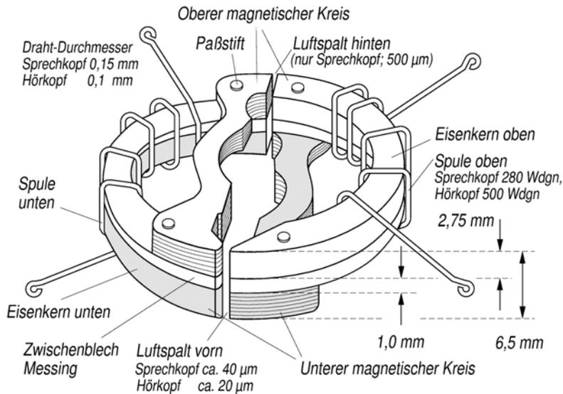
Fig. 7: Schematical representation of stereo magnetic head as used by RRG (developed by Eduard Schüller, AEG)
