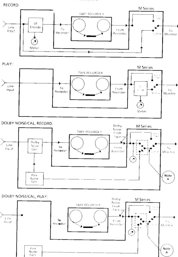
Note A: Cat No. 280 modules before serial number 456 have the meter connected to the unitput of the Auto-Compare switch. Boards stamped 456 and above have the calibration meter connected as drawn. The result is that when an early generation Cat No. 280 m used, the calibration meter will lead the reference noise/Dolby Noise sequence, while with later generation boards, the calibration meter will always read the Dolby Noise from the recorder.
