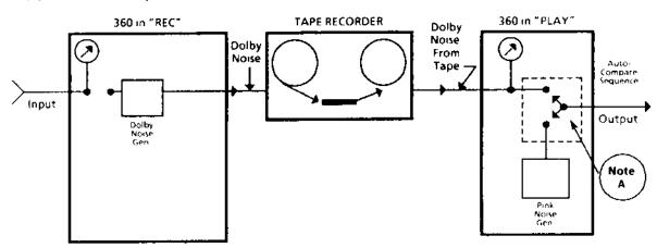
**Note A:** Cat. No. 280 modules before serial number 456 have the playback meter signal connected to the output of the Auto Compare switch. Boards stamped 456 and above have the calibration meter connected as drawn. The result is that when an early generation Cat. No. 280 is used, the calibration meter will read the reference noise/Dolby Noise sequence, while with later generation boards, the calibration meter will always read the Dolby Noise from the recorder.
