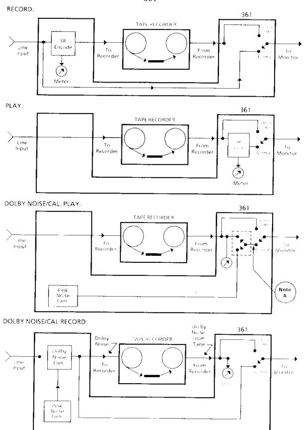
**Note A:** Cat No 280 modules before serial number 456 have the meter connected to the uniquit of the Auto Compare switch. Boards stamped 456 and above have the calibration meter connected as drawn. The result is that when an early generation Cat No 280 is used, the calibration meter will read the reference noise/Diciby Noise sequence, while with later generation boards, the calibration meter will always read the Dilby Noise from the recorder.
