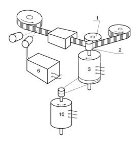
Fig. 6: Weber and Augustin: Synchronisation between film and magnetic tape by means of "sprockets" printed on the back of the tape<sup>31</sup>
