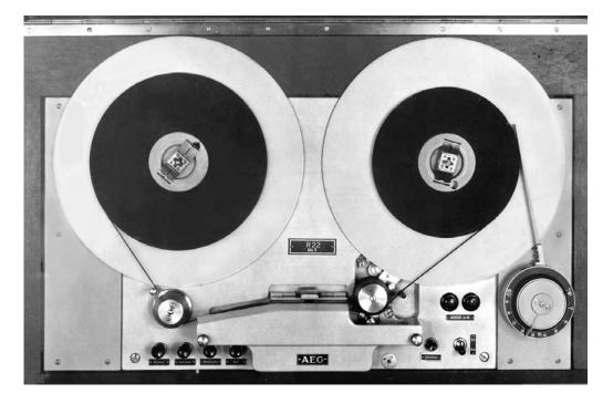
Fig. 5: Magnetic tape recorder "Magnetofon R 22" of about 1939, customer built by AEG for RRG (German Radio). Tape speed 77 cm/s (approx. 30 ips), tape width 6.5 mm (approx. ¼"), playing time with 1.000 m of tape around 22 min
