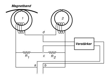
Fig. 2: Weber's experimental circuit for noise reduction via negative feedback: 1 active magnetic recording head, 2 "dummy" head; Magnetband = magnetic tape; Verstärker = amplifier. The bridging voltage occurring at d and c – the difference in voltage between heads 1 and 2 – would be amplified and act as a negative feedback, thus decreasing the tapeinduced noise in the recording process
