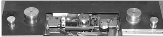
Figure 10. Controlling tape tension: A reel of Melody 169 that was recently transferred was done with a modified Studer A810 with the erase and record heads as well as some guides removed. Source: the author.
